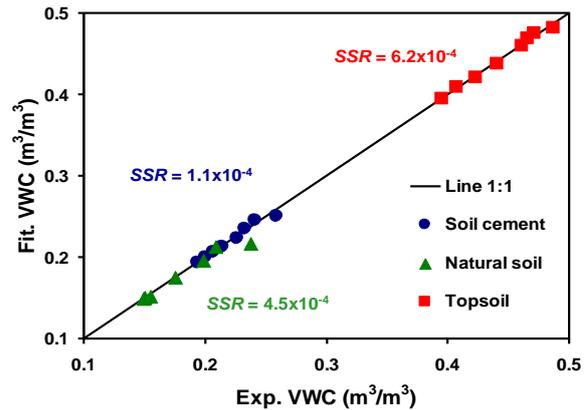
Fig. 4. Relationship between the values of volumetric water content (VWC) measured by experimental form and the calculated via a Fit program based in VG-model.
