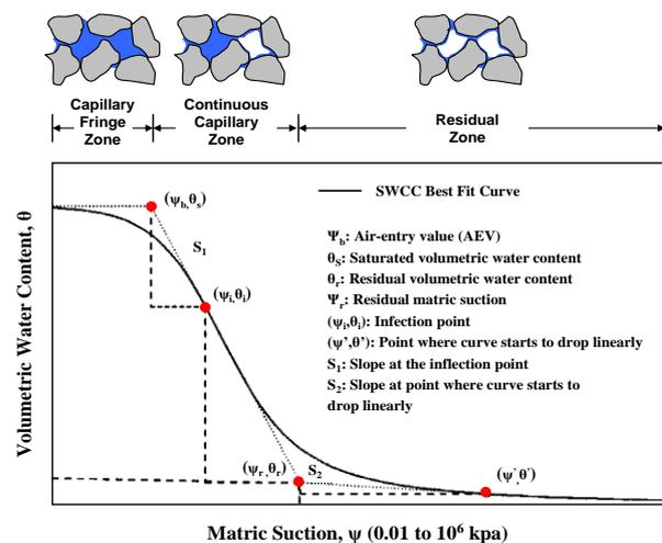
Fig. 1. Soil Water Characteristic Curve form and its variables (modified from Zhai and Rahardjo, 2012).
