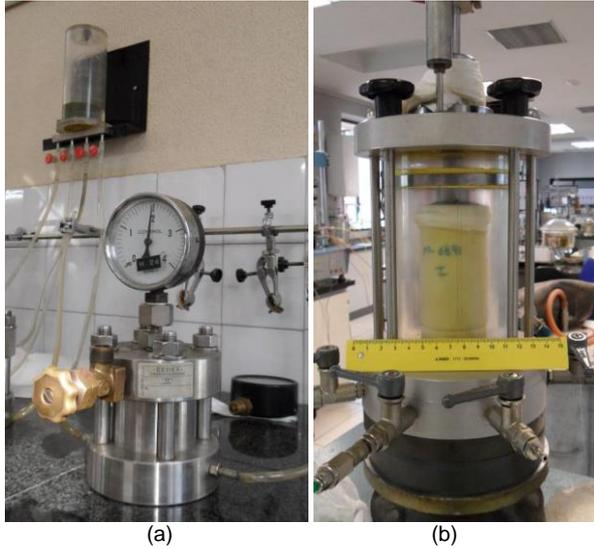
Fig. 2. Equipment for measurements of the hydraulic properties: (a) Pressure cells apparatus to measure matric suction based in axis translation technique, and (b) triaxial cell apparatus to measure saturated hydraulic conductivity.
