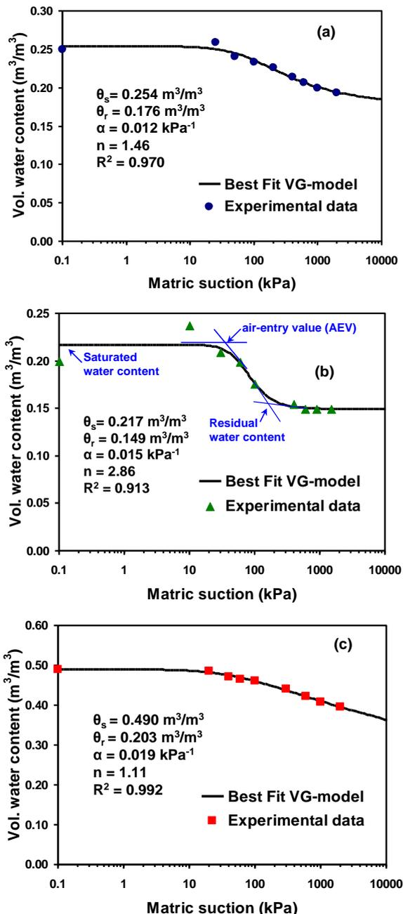
Fig. 3. Drying SWCCs and fitting parameter of VG-Model for: (a) Subgrade improvement, (b) subgrade of natural soil, and (c) topsoil.
