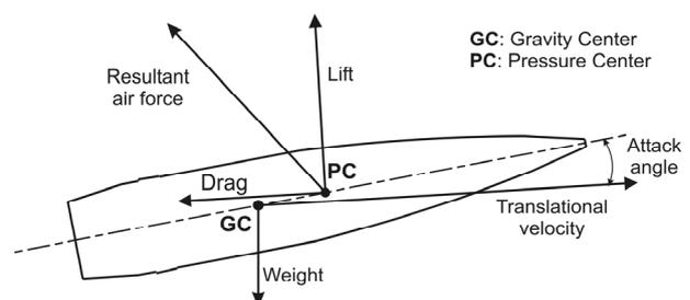
Figure 2: Sketch of aerodynamic forces acting on a projectile.
