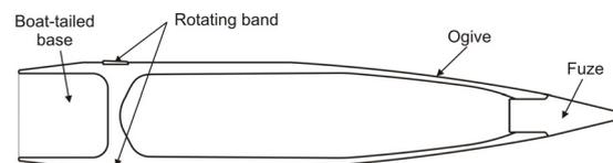
Figure 1: Relevant projectile parts.
